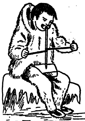
STRAP DRILL USED BY ESKIMO OF ALASKA
