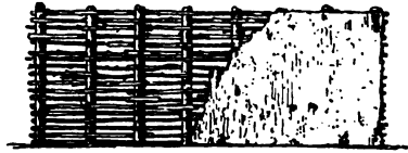
HOUSE CONSTRUCTION, MOUND BUILDERS. PLASTERED WATTLE WORK. (THOMAS)
