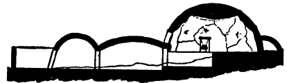
SNOW HOUSE OF CENTRAL ESKIMO. a, FRONT VIEW; b, GROUND PLAN; c, SECTION. (BOAS)
